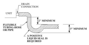
The condensate drain line must be at least 3/4 NPT, for each unit. Precautions must be used not to over tighten the adapter at the drain pan connection, this precaution will prevent damage to the plastic drain pan. A joint compound should be used to prevent leakage and act as a lubricant.
